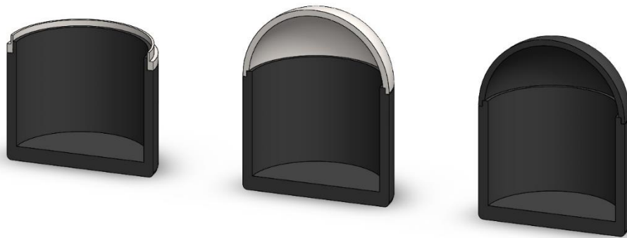
Schematic representation of the evaluated closure concepts. (Image: Nagra)
